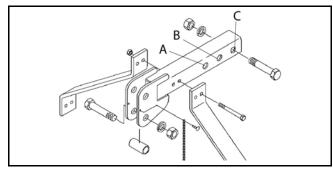
Figure 2. 3-Point Hitch Adjustment Positions
